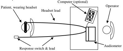
The patient is seated in front of the desk facing away from the operator. The patient wears a headset (see Section 4.3) and responds to test stimuli by use of a hand-held switch which is also connected to the instrument.
